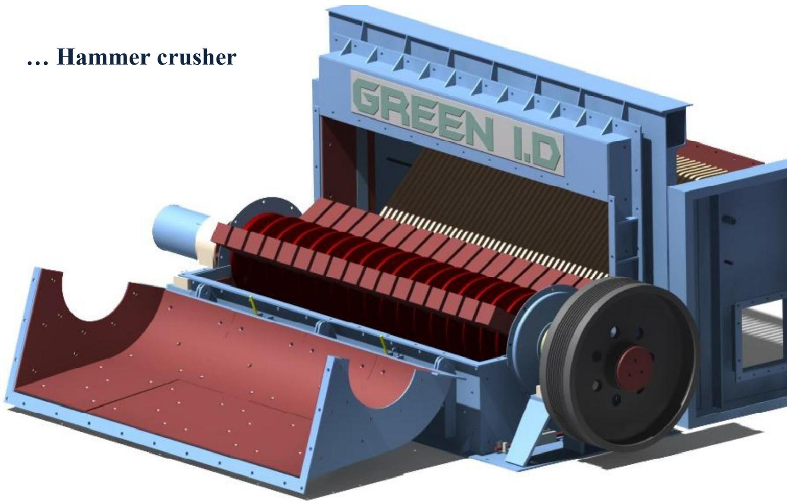
The cement clinker burning process produces agglomerated balls of clinker which may be so large as to make their further passage from the kiln for storage or grinding extremely difficult. To avoid such complication, these balls are removed at the clinker cooler outlet and reduced in size by clinker crushers before being returned to the main clinker flow.
