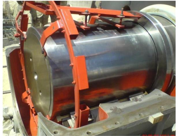
They are dimensioned to ensure they are not affected by any types of load resulting from various operating conditions. However, in the event that it is necessary to straighten a bent shell of a three-station kiln during operation, the system is equipped to do so. The extremely robust and solid construction of the bearing arrangement, with double slide bearing blocks which remain aligned, is designed to ensure that the roller stations have a centering effect on the kiln.
