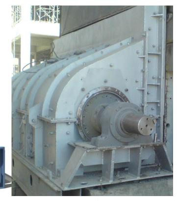
GREENID clinker Crushers are equipped with adjustable jaws which can not only be set at the required degree of crushing, but can also be adjusted to compensate for hammer wear.
