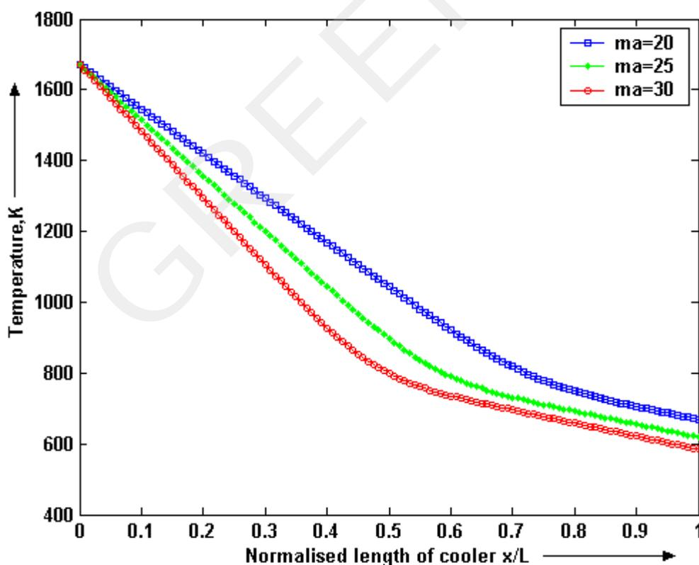
**Figure. 13** “Variation of average caloric temperature of the clinker along the length of cooler at different mass flow rate of air”
