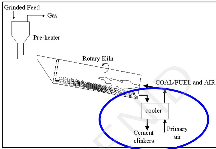
**Figure 1:** Schematic of Cement manufacture
