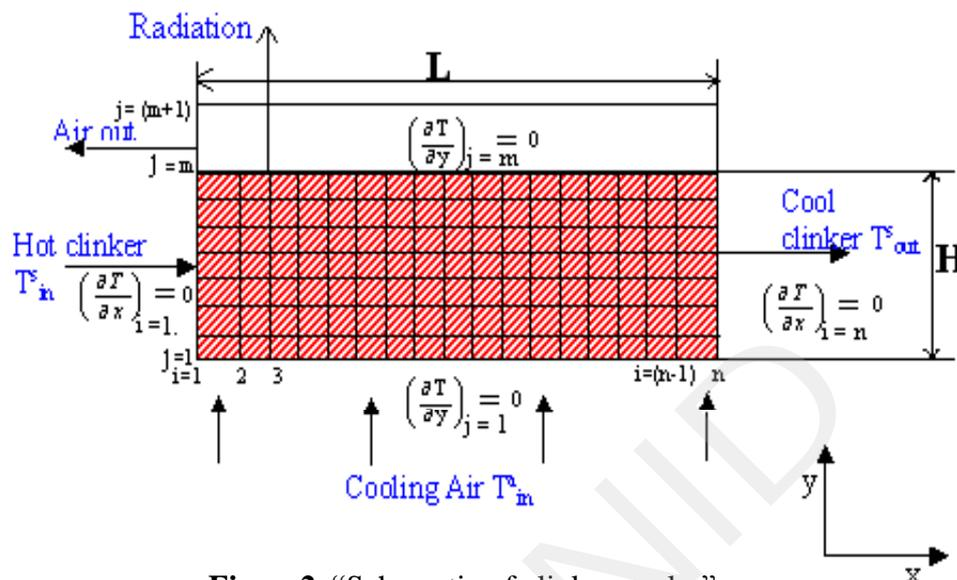
Figure2. "Schematic of clinker cooler"
