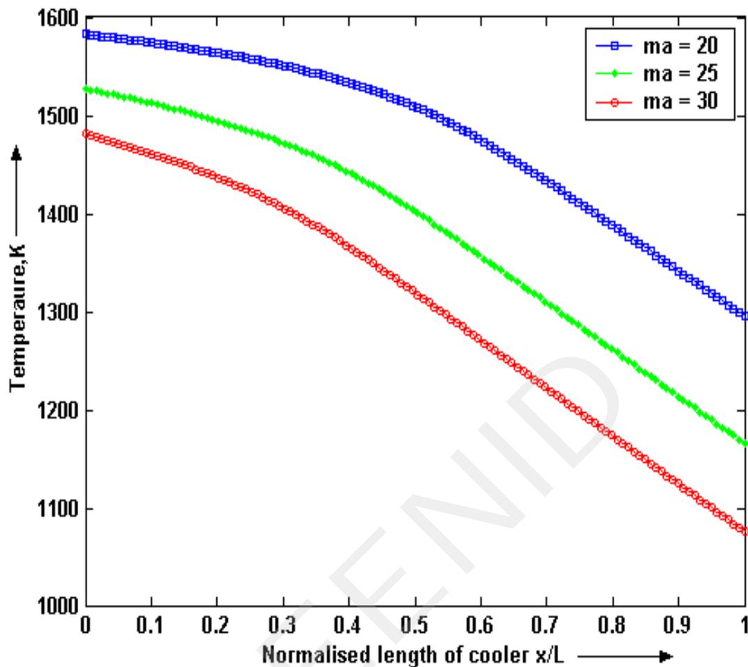
**Figure . 14** “Variation of average caloric temperature of the clinker along the length of cooler at different mass flow rate of air”
