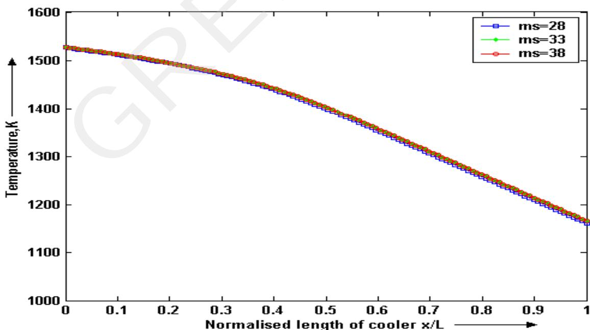
Figure. 12 “Variation of air temperature in free board region along the length of cooler at different mass flow rate of solid”
