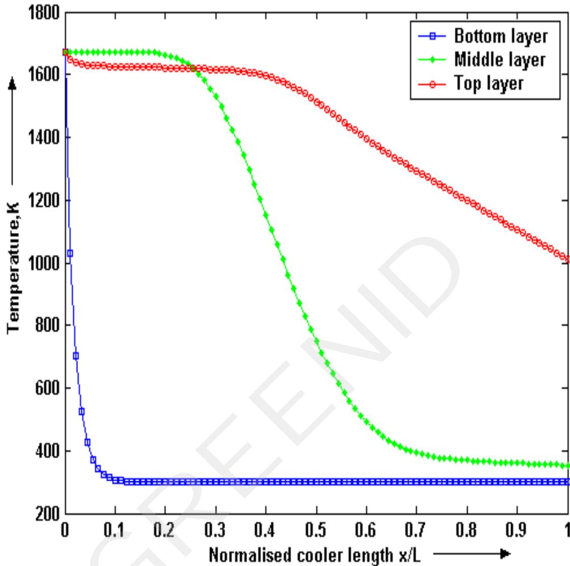
**Figure: 7** “Clinker temperature variation against cooler length at various heights”
