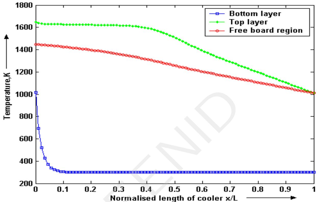
**Figure 9** “The temperature variation of air along the length of cooler”
