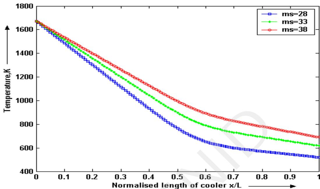
Figure. 11 “variation of clinker temperature along the length of cooler at different mass flow rate of solid”
